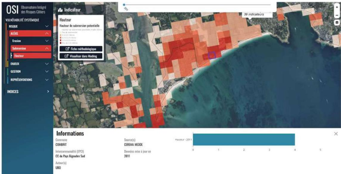
Figure 20: Example of marine flooding indicator on the OSI web-platform interface (Île-Tudy, Brittany, France).
